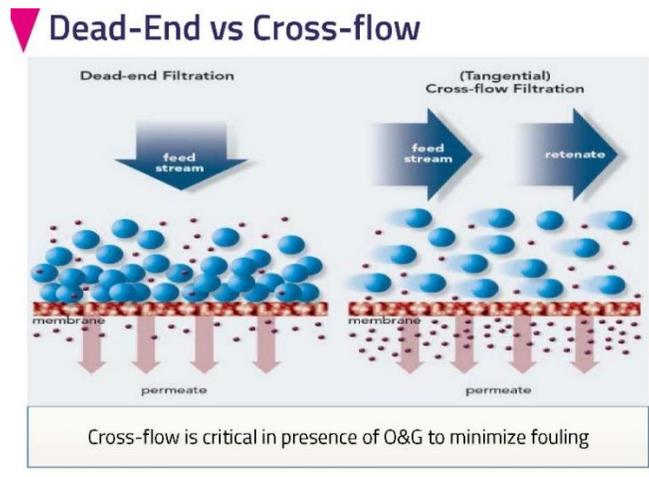
Cross flow systems employ sweeping forces at the membrane surface to reduce fouling as the permeate is removed resulting in the stream becoming more concentrated for batch processes as it is recycled and filtered to its maximum concentration factor.
