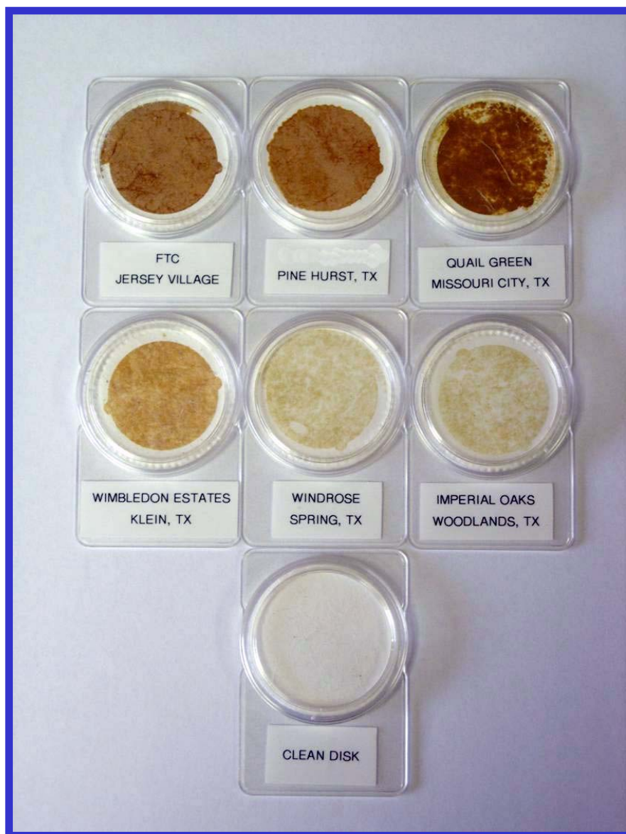
Figure 1. Solids Captured from 2.6 gallons of water (10 liters) Sample Contaminants Range from 0.2 mg/l to 0.5 mg/l.
